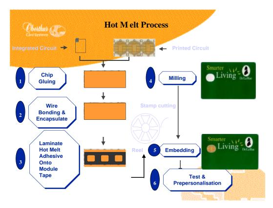
A serial number is next programmed into the chip and all cards are electronically tested. Random ISO 7816 sample tests are performed on each manufactured batch of cards. The smart card is then pre-processed to create a so-called "virgin" smart card. Finally, a file is prepared of the serial numbers of all smart cards produced in a given production run. The embedding phase usually takes 3 weeks.
